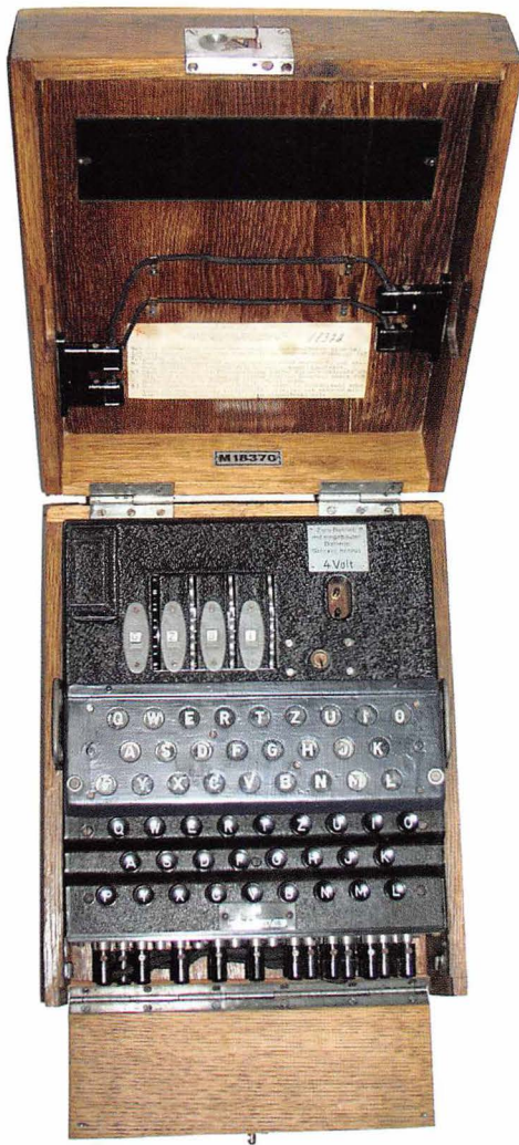
An Enigma machine was used to encrypt military messages in World War II. It was Al-Kindi in the ninth century who laid the foundation of cryptography.
